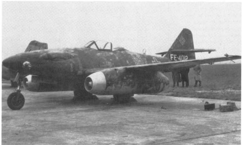
A Me 262 A-1a/U3, FE 4012, with the stream lined fairings over the camera. Photo taken September 30, 1945. (USAF Photo)
