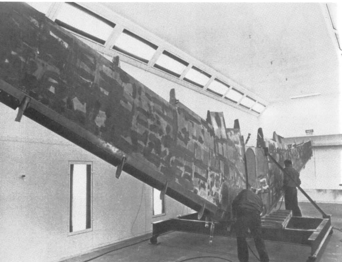
The exterior surface of the wing was sanded and treated for corrosion.
