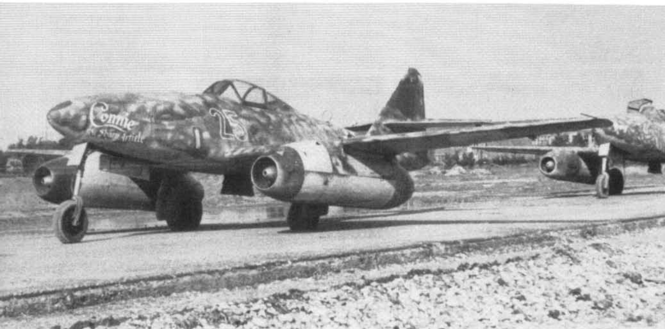
Lt. Roy Brown's plane, "Connie The Sharp Article." These names were not chosen by pilots of Watson's Whizzers. Note bulge on nose which faired in the RB 50/30 cameras of this Me 262 A-1a/U3.
