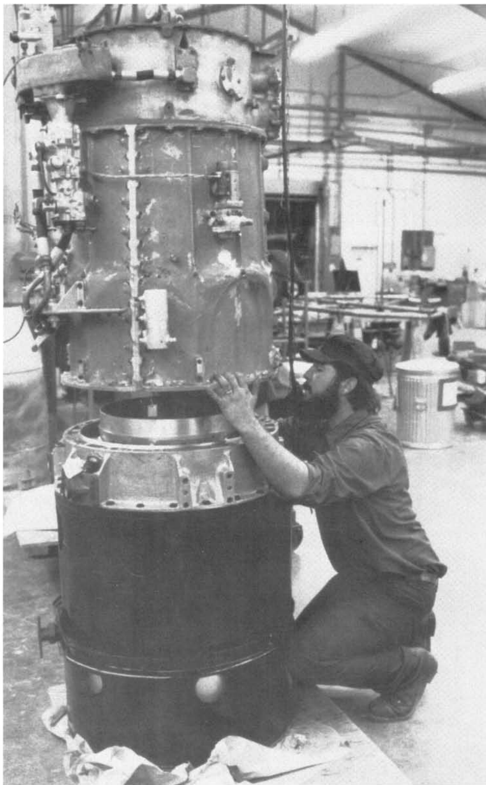
The engine was torn down, refurbished, all corrosion arrested, and then built up again. This was Bill Reiss' first important assignment at Silver Hill, and he went all out to do a first rate job.
